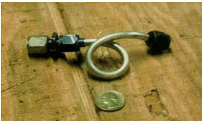
when finished. Then install the sleeves and nuts and flare the tubing ends. Then install unions on both ends and cap one end with an AN 929 cap. Fill the tubing completely with bead blast material (sandblasting sand will work) and cap the other end with the same part number cap. Then you can bend the tube any way you want and it will not kink. After bending, just empty out the material and blow clean. I bent the piece of tubing in the picture around a broom stick.
