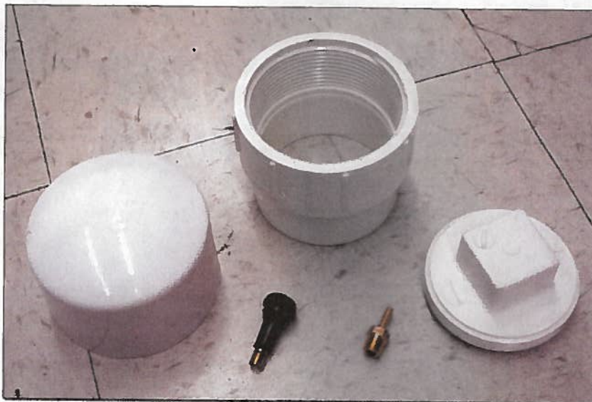
Main components from the hardware store: 3-inch PVC end cap, clean-out adapter and screw-in end cap, tire Schrader valve, and 1/8-inch pipe male to 1/8-inch barbed brass fitting.
