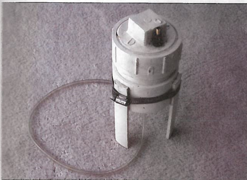
The finished product. Note the Schrader valve attached to the screw-in cap. Strips from a piece of 3-inch PVC pipe were used to make the legs.
