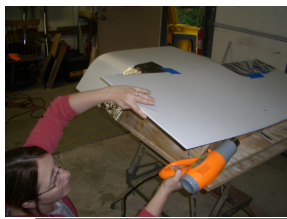
Belly Panel Form Lay-up with Finished Product
